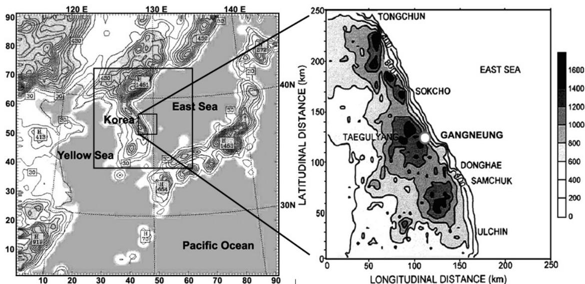
**Fig. 1.** Topographical features in the vicinity of Korean peninsula in three different domains (horizontal resolutions of 27 km, 9 km and 3 km, respectively) for numerical simulation using WRF-2.2 model (left) and the mountainous coastal region surrounding Gangneung city (37°45N, 128°54E; 20 m above mean sea level) and Mt. Taegulyang (860 m) in a fine-mesh domain (horizontal resolution of 3km) (right).
